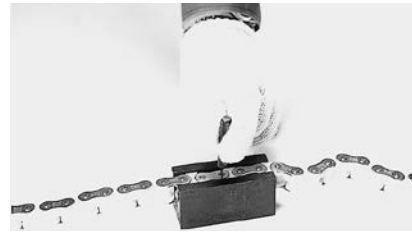
Figure 16: Disconnecting Poly Steel Chain
