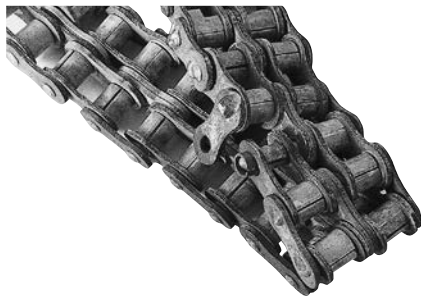
Corrosion of Stainless Steel Drive Chain
