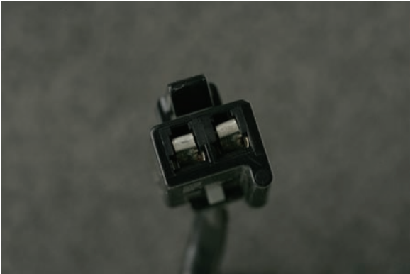
Metri-pack 280 Series Female Sealed
