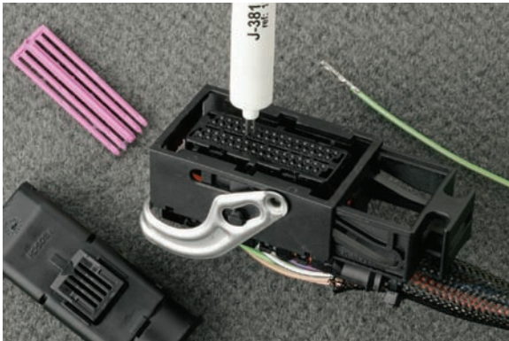
Terminal release tool inserted into connector
