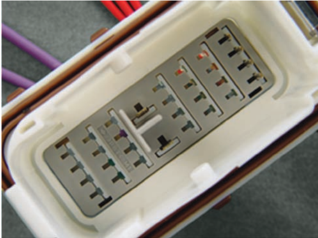
Connector half houses male terminals.
