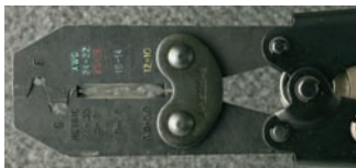
CRIMPER - F&G - Sealed Splice Part #: 12085115 J-Number: J-38125-8
