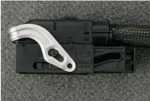
Connector w/ .64 round terminal
