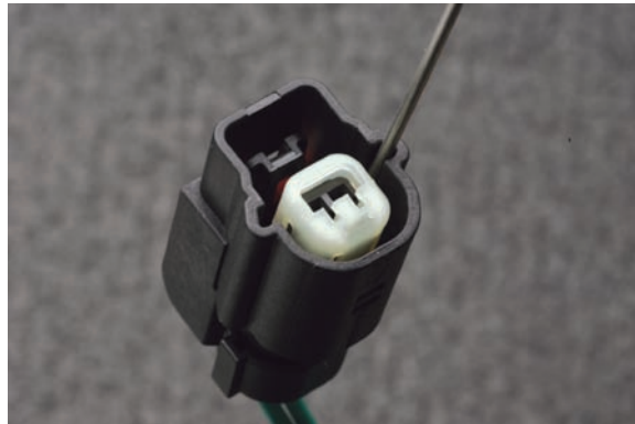
TPA is pulled up into the "preset" position using J-38125-216. Do not remove the TPA.
