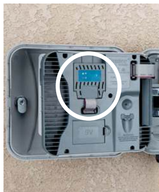
PC-WIFI Wi-Fi accessory for Pro-C Controllers, managed by Centralus Software page 104
