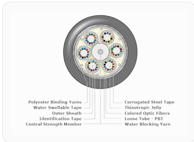
ARMORED DUCT OFC — LAYER DETAILS
