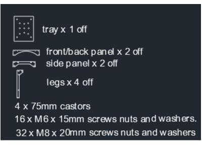
Attach legs x4 to shelf using M8 screws, nuts, and washers.
