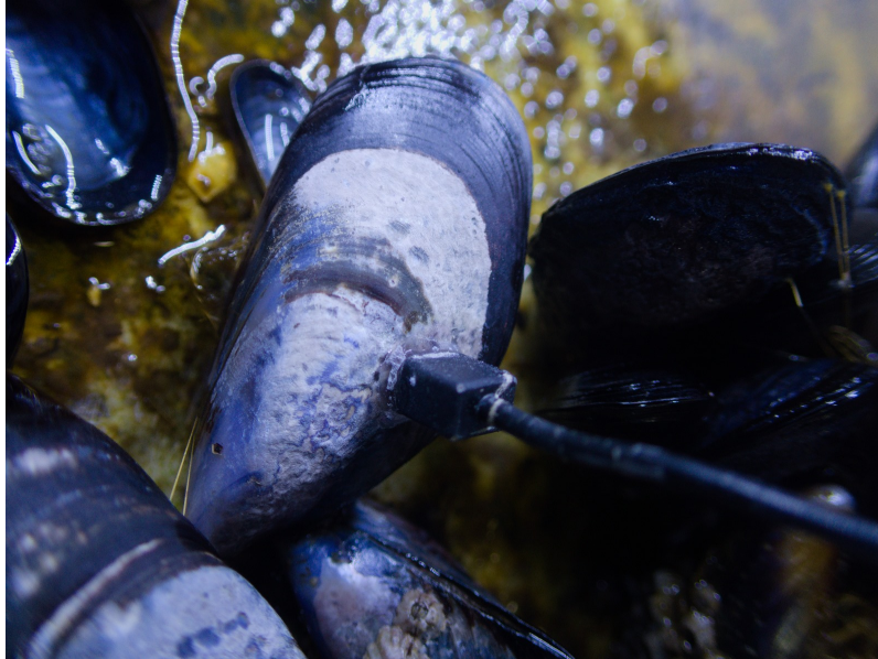
Figure 2: IR CNY70 sensor glued on a mussel with cyanoacrylate (superglue).
