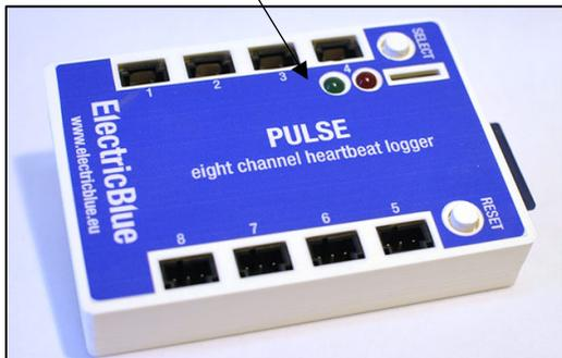
Fig. 6. The two LEDs and the slit through which the micro-LED strip shines through.
