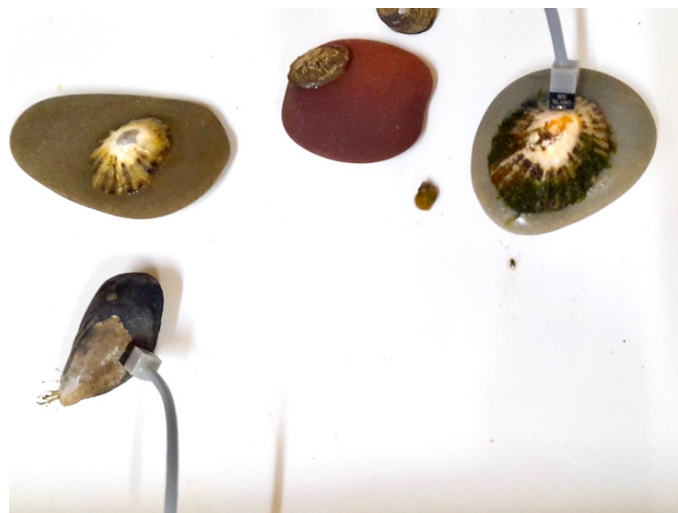
Fig. 7: A CNY70 sensor glued to a Mytilus galloprovincialis (left), and another glued to a Patella vulgata (right).
