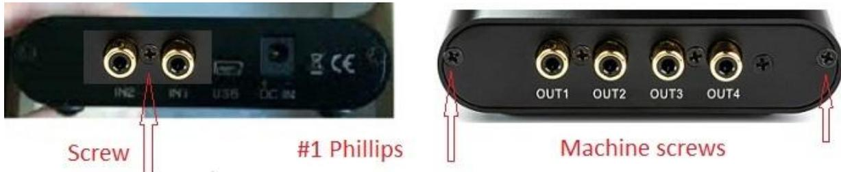
Only three screws need to be removed to take the cover off .
