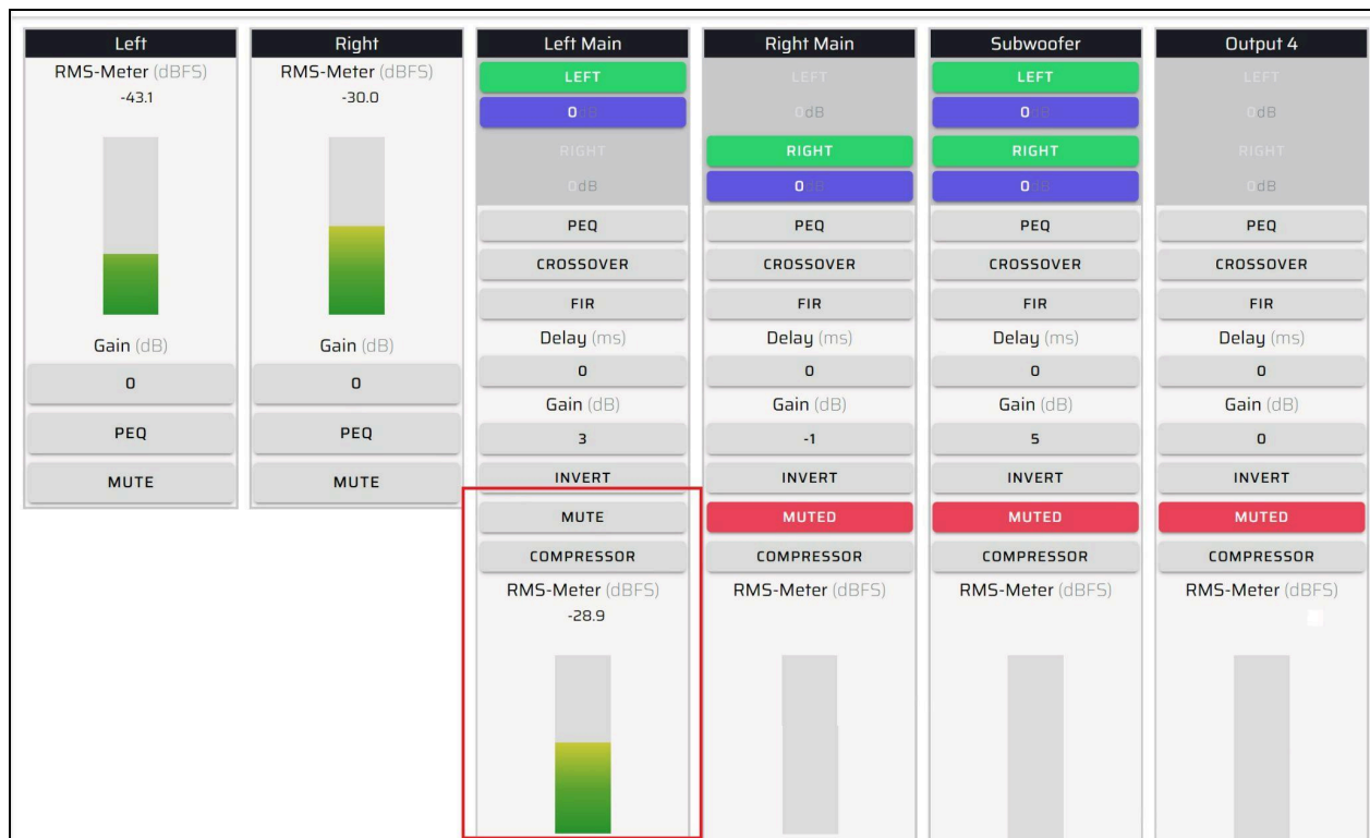
Diagram 5. Using miniDSP Device Console, you can selectively mute the left speaker, right speaker and subwoofer. Here we are measuring only the right speaker.
