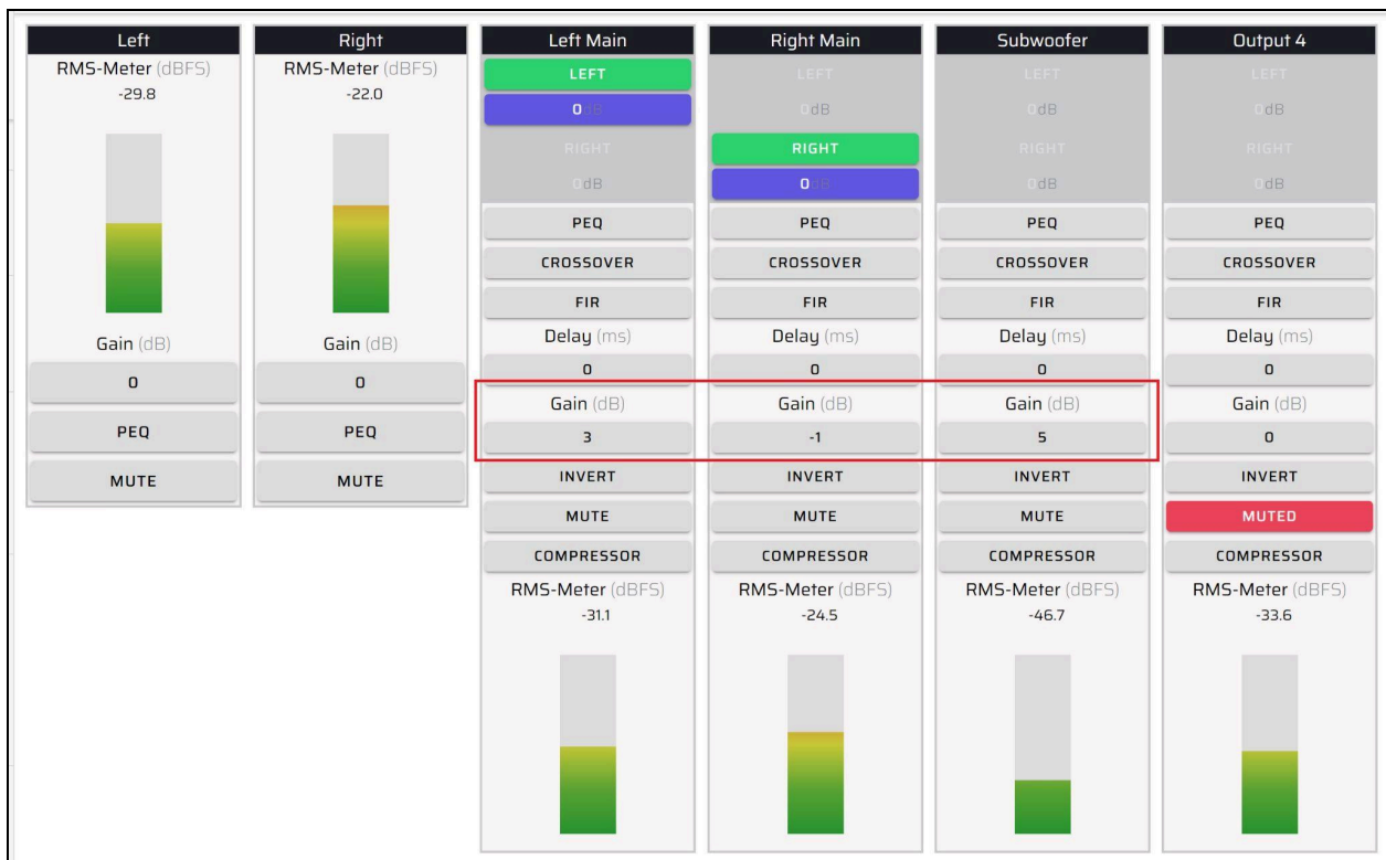
Diagram 10. Here we use the miniDSP output page to adjust the output amplitude values
