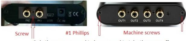
Only three screws need to be removed to take the cover off . Make note of which screws go where, as there are two types.
