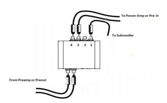
If you have a receiver or integrated amplifier with a pre-out / main in loop, you can insert the EQ901B as shown below.
