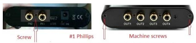
Only three screws need to be removed to take the cover off.
