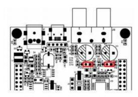
**0.9 Vrms position.** The maximum input signal voltage allowed before clipping the A/D converter is 0.9 Vrms. This position is typically used when the EQ901 PS is connected between a pre-amplifier and a power-amplifier.
