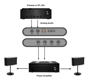
If you have a receiver or integrated amplifier with a pre-out / main in loop, you can insert the EQ901B as shown below.
