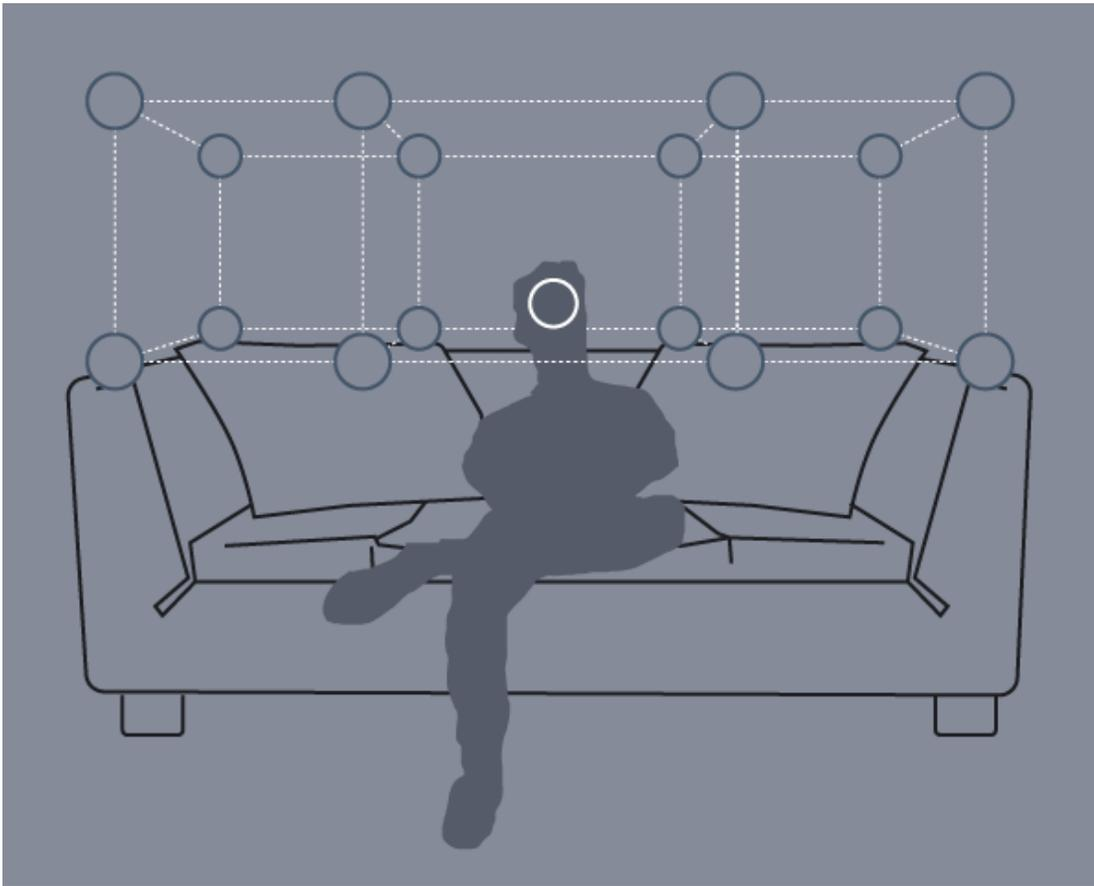
Diagram 13. Three dimensional space and recommended microphone positions
