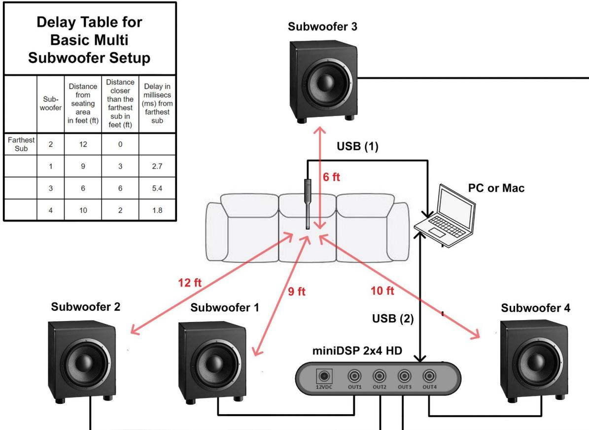
Diagram 6. Delay table for basic multi-subwoofer setup
