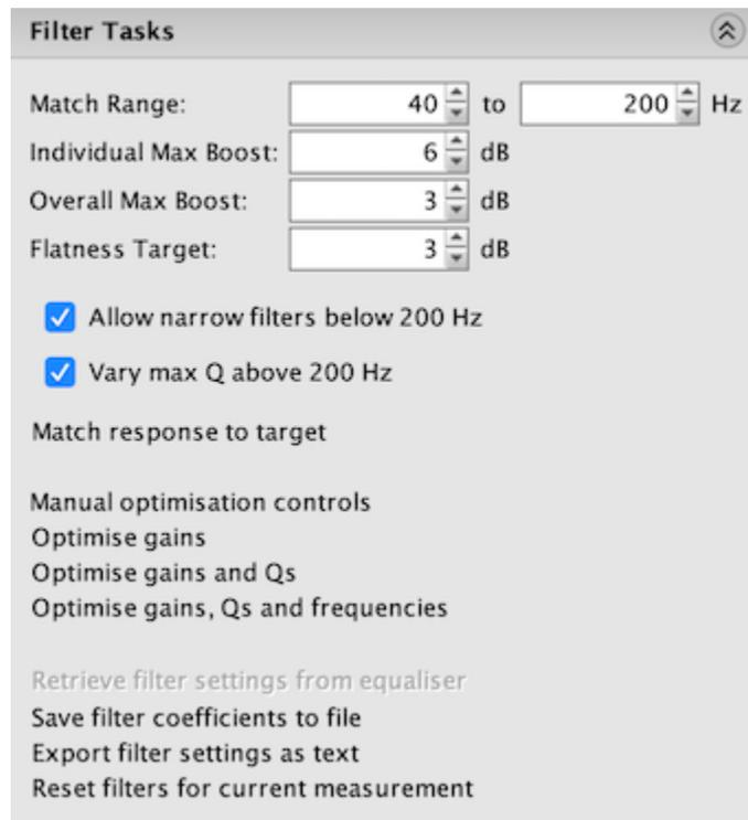
Diagram 15. Setting parameters for REW inverse filter generation
