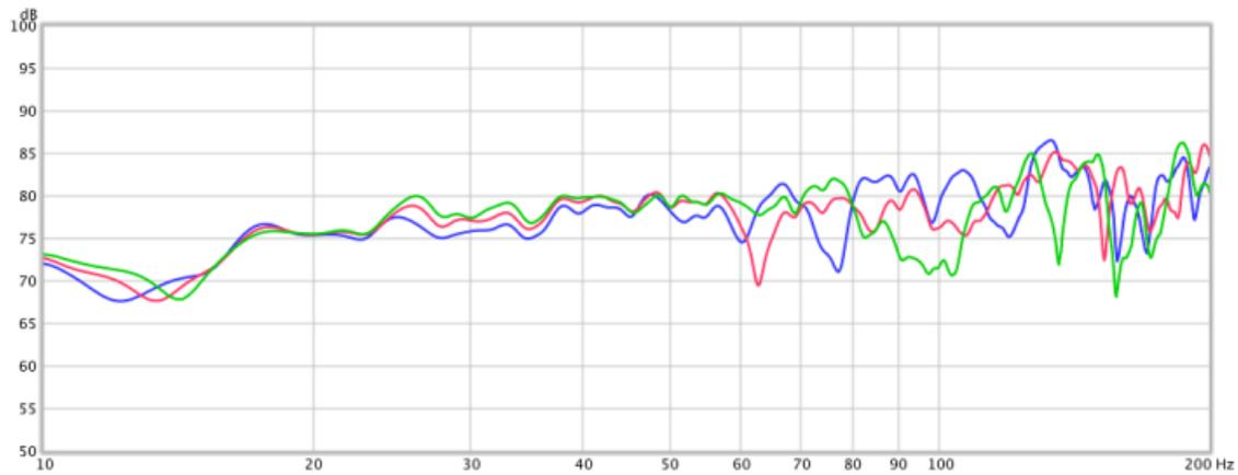
Diagram 12. Three subwoofer relative amplitude overlay plot
