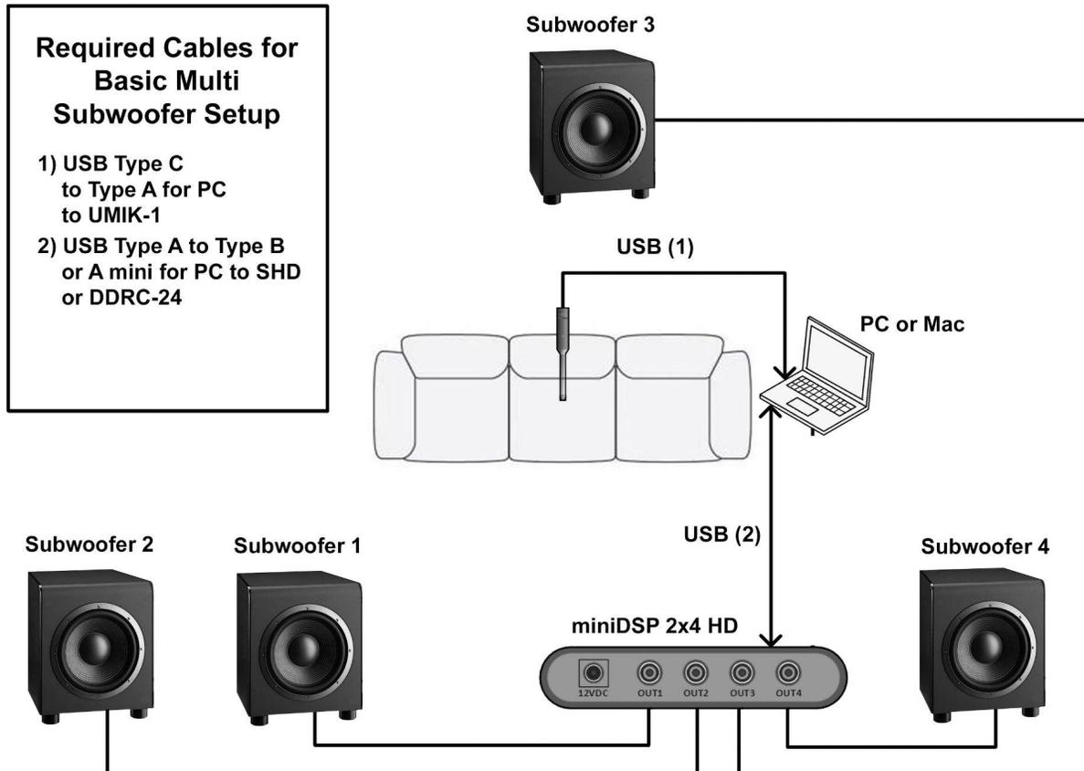
Diagram 2. Required connections and cables for system setup, measurement and correction
