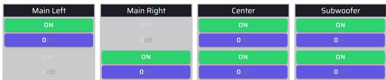
Diagram 4. Routing matrix set for 3.1 stereo for home theater audio
