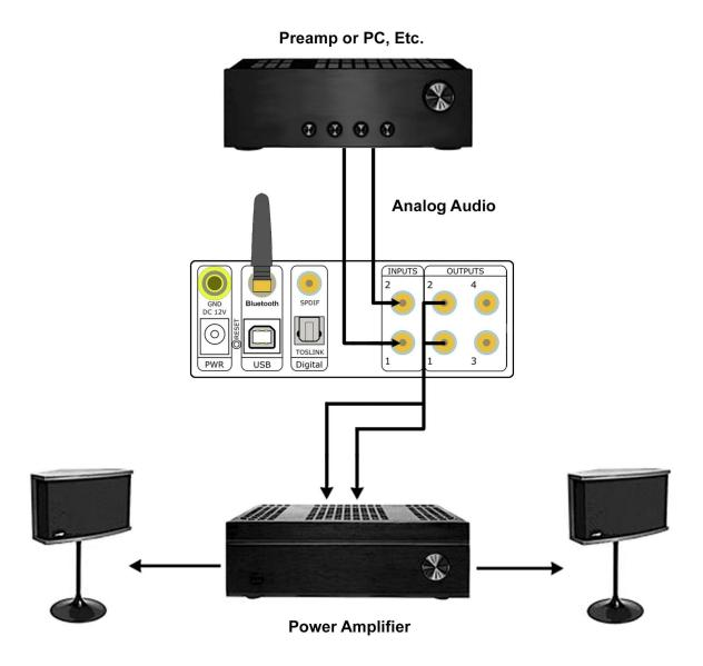
If you have a receiver or integrated amplifier with a pre-out / main in loop, you can insert the EQ901 Platinum as shown below.
