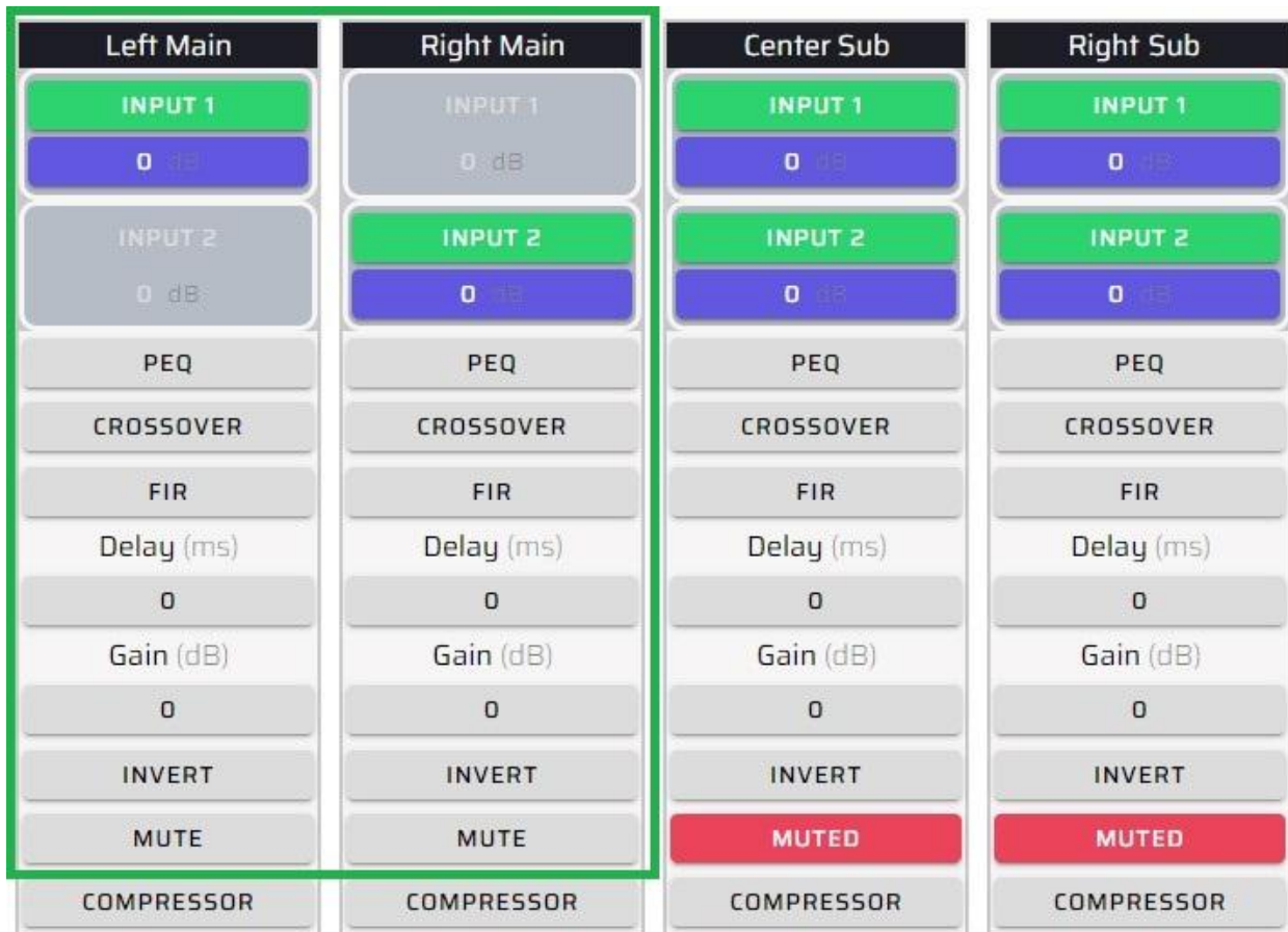
Diagram 8. Measuring the delay of the right main speaker relative to the left main speaker (timing reference)
