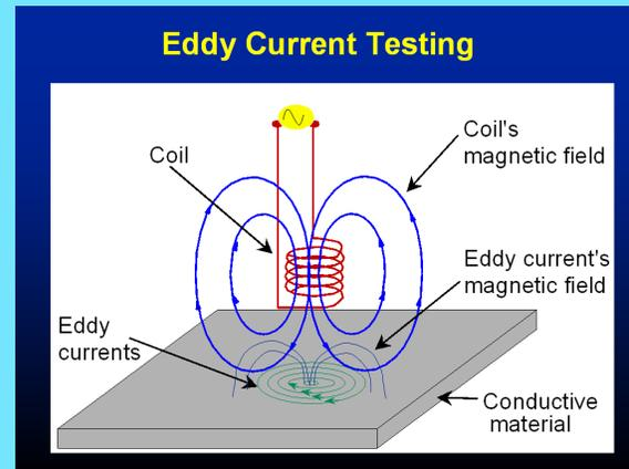
Measuring the magnetic field variation induced by eddy current with a probe coil, can be inferred from the test size and phase change in eddy current. And then get the information about the changes of electrical conductivity, defects, material conditions and other physical quantity or defects. But because the eddy current is the alternating current, which has the skin effect, the detected information can only reflect the condition of the specimen surface or near surface.
