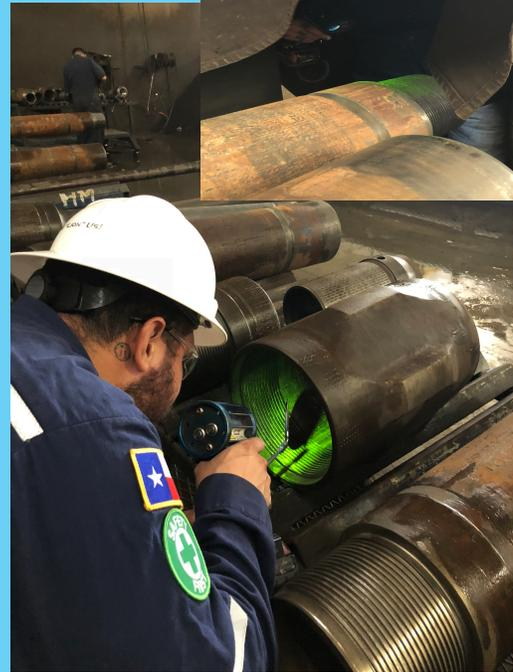
WET MAGNETIC PARTICLE INSPECTION
