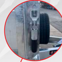
'Silent Sides': Spring loaded flip latches on all drop sides prevent undue movement and noise
