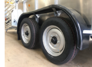
Wheels: bigger surface area tows better in fields and gives extra stability on the road. Less rolling resistance, giving a better fuel efficiency & reducing the pull on the towing vehicle.
