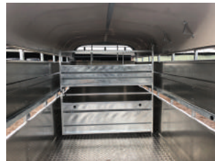
Internal dividing gate with multiple hanging locations.
