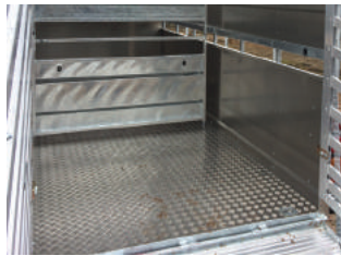
30mm timber floor with a one piece, fully sealed 3mm aluminium tread plate floor covering.
