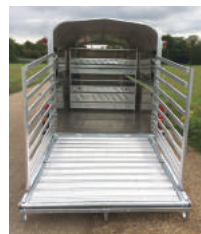
Reinforced loading ramp.
