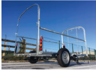
Chassis made from angle iron with a fully welded frame for maximum strength and endurance.
