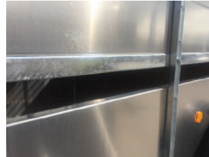
Incorporated box section for strength and reinforcement.
