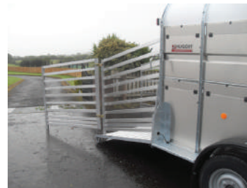
Additional pair of loading gates.
