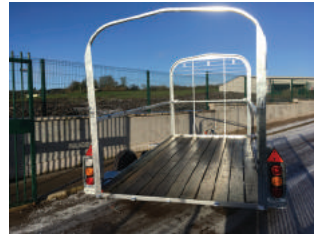
30mm preserved timber floor with aluminium treadplate for a fully sealed finish.
