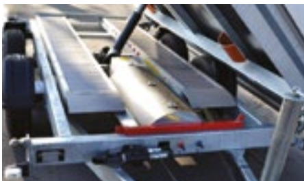
■ Emergency hand pump
