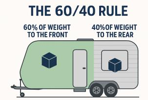
Packing your caravan properly is essential for safe towing. Aim to place about 60% of your load forward of the axle, keeping heavy items low and close to the axle or slightly forward. Avoid placing heavy gear at the rear, as this increases sway risk. Use the 60/40 rule as a guide, and remember lighter items can be placed higher if required. Maintain a balanced setup for a smoother, safer towing experience.
