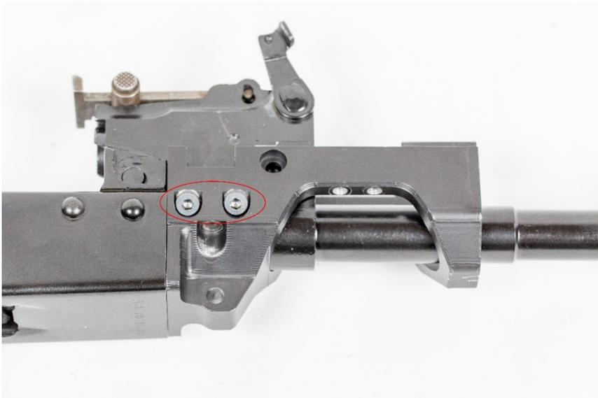
5. Loosen gas tube screws and install “top front rail” by turning 90 degrees to clear the rear sight.
