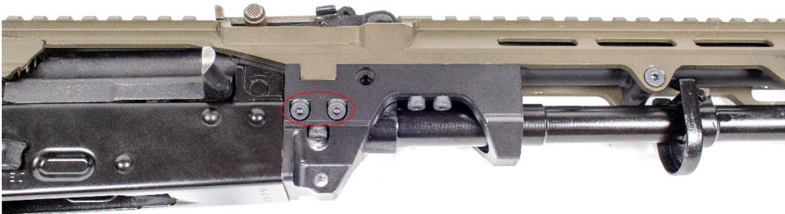
10. Slide "handguard" into position making sure the MLoc hardware in the front indexes into their slots and the main bolt in the rear is lined up then tighten.
