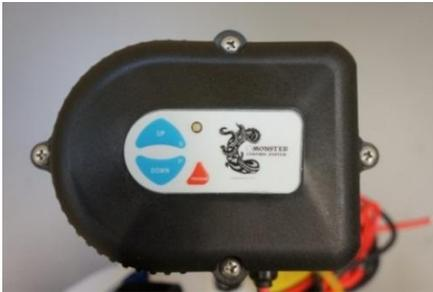
5. Remove the motor cap leaving membrane switch's ribbon attached.
