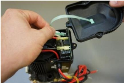
6. Connect the USB Cable to the motor's board and your computer.
