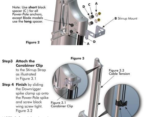
NOTE: Before tightening wing screw, make sure to keep Downrigger cables tight as shown in Figure 3.3
