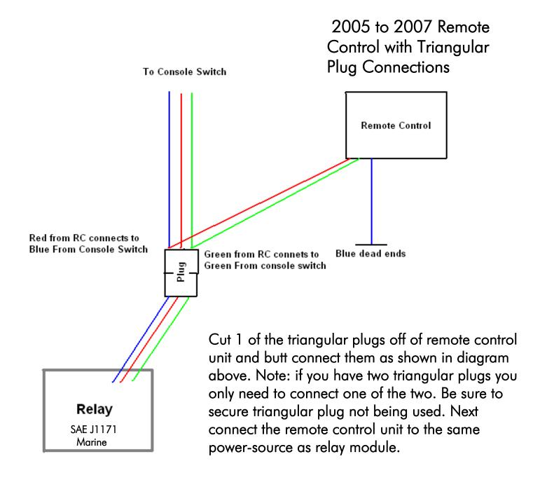
Note: Be sure to mount Remote Control box up on a wall with wires exiting bottom.
