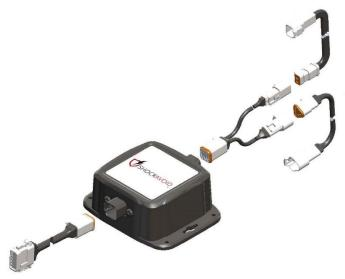
**Step 3:** At an appropriate concealed and protected location, connect the 2-Pin cable that you just ran our of the cab to the Harness "T" Assembly.
