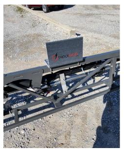
You must use extreme care in planning and mounting the sensors and brackets. Since most brackets fold when racked, be sure that where you place the sensors, neither they or the sensors conflict with or make contact with other boom parts when racked or in the process of folding to rack the booms.
