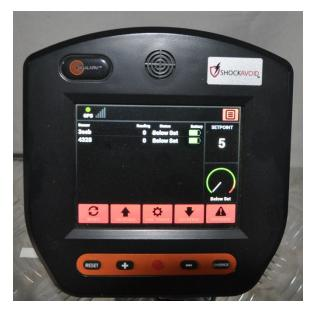
You'll see the codes for the respective sensors. If not, touch the "Home" button on the upper right hand of the touchscreen. A new page will appear, showing several different selections. Touch the "Manage Sensors" button. The system will ask for a pass code. Enter 0000 (zeros). A new screen will appear. You should see the two sensors codes you wrote down on the list. If you do, then you have sufficiently charged active sensors installed. If you do not, please call us for trouble shooting
