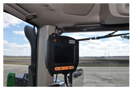
Mount the Control Console to the windshield pillar or side bracket.
