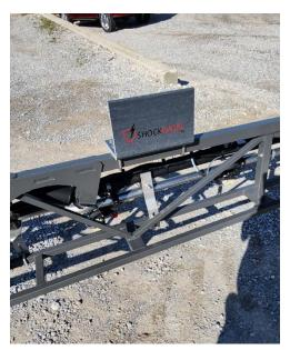
The fiberglass brackets will fit most boom applications. We have them pre-drilled to accommodate u-bolts for various booms. The brackets are very low maintenance, and you can modify them if needed for your specific application.
