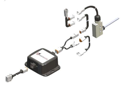
**Step 5:** Connect the **Siren/Strobe** to the remaining connection from the **Harness "T" Assembly** using a provided **2-Pin Extension Cable**.
