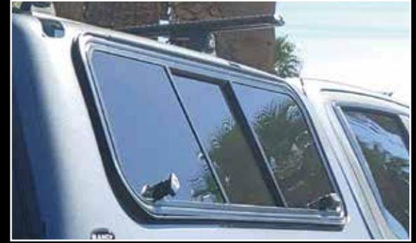
Optional side Window with Slider provides ventilation without opening the Window
