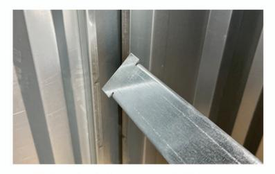
**3.3** Twist the shelf arm at around 45 degrees to enable it to slot into the shelf upright. Now twist the shelf arm, sometimes a small tap is required to locate the shelf arm into the final position. If you need to remove or reposition the shelf arm at anytime, twist the shelf arm in the opposite position and lift upwards.
