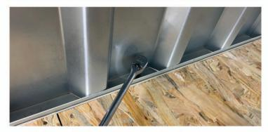
**1.20** Now fix the side panel to the chassis using M8 and M10 bolts and washers.
