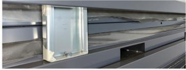
**1.12** Whether or not you need to move the parts to a different location, the container now needs to be unpacked. Unbolt the four metal retaining plates using a 19mm socket wrench and also unscrew the lifting eyes. The retaining plates are not required for assembly, so dispose or keep if you intend to re-pack the unit at a later date.
