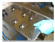
Turn off all valves. Inspect gun and clean off any remaining paint with flow thru brush.
