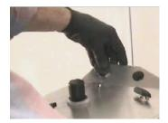
Press Blaster Button for 10 –15 seconds. This will flush paint gun internals with high power stream.
