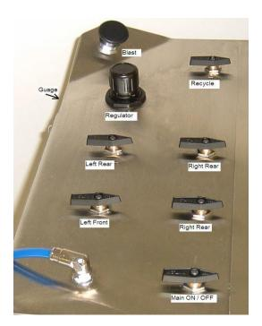
Always turn Main ON –OFF valve OFF whenever system is not in use.
