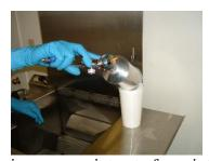
Drain excess paint out of gun into a cup or other container as per Material Waste minimization plan.
