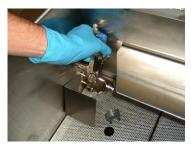
While keeping the paint gun upside-down, place trigger clip over handle and trigger to keep paint gun fully open. Place gun upside down on left wash nozzle in back corner of the basin. Gun should be placed loosely on wash nozzle so that some fluid goes into the gun while some leaks around and cleans the treads. Position gun down so stream will spray out safely. Turn on LEFT BACK fluid valve.
