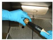
While the solution is cleaning gun and cup, clean air cap and cup lid.
