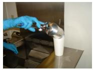
Drain excess paint out of gun into a cup or other container as per Material Waste minimization plan.
