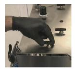
Start pump by turning on MAIN ON/OFF valve on front of control panel
