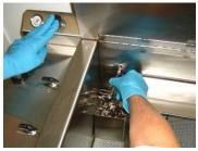
Hold the gun firmly on left gun mount with your right hand and press the solution BLAST button on back of control panel with your left hand for 8 seconds. This will propel solution through the gun with significant force for thorough cleaning. If paint in gun was allowed to dry or if you are cleaning a tough primer, you may need to hold the BLAST button a few seconds longer.
