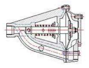
Automatic air exhaust valve, suitable for installation in a raw sewage lift, with interconnection of return to the suction pit, closing through diaphragm and opening by spring, with device for adjusting the spring tension and threaded connections.
