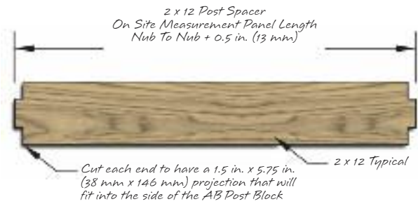
Figure 4: Post Spacer Jig
