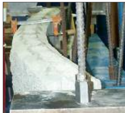
Top bond beam deflection.
