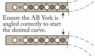
Ensure the AB York is angled correctly to start the desired curve.
