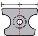
Modify the block down the center of the hole.
