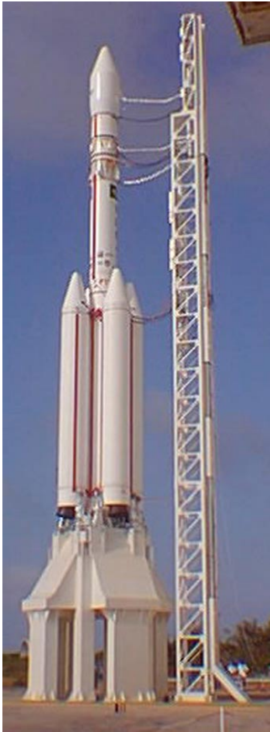
Best available photo of VLS, vehicle 1. The red lines are external conduits. The protuberances in the first ring below the payload section are antennae; the second ring consists of solid rockets for the roll control system. Note latticework at the top of stage 1 and a ring of what appear to be decals above that.
