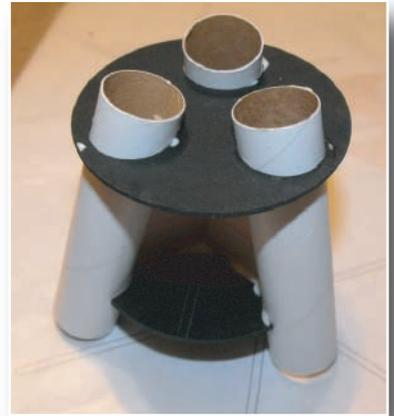
distance and gave the Motor Tubes a solid structure to be mounted to. Using yellow carpenter's glue, I glued the three balsa supports to the Centering Rings then added the Motor Tubes and Thrust Rings. I tied a length of Kevlar around one of the Motor Tubes just behind the forward Centering Ring and threaded it up in front of the Centering Ring. With the glue still wet I made sure that the three Motor Tubes were aligned properly and set it aside overnight to let it dry.
