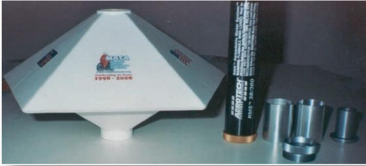
This new hardware was the basis of the CINCO flights. Since the CINCO can fly any 38mm motor with an average thrust of 50N to 250N, that covers G,H, and I motors. With the 38/360 RAS Special, I could cover all the range of this rocket with just one hardware unit. Also, that kept the CG forward.
