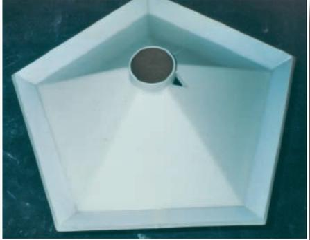
I had placed the motor tube just outside the Top section to provide room for an epoxy joint. I just decaled the Top and used Acrylic sealer for the top coat.
