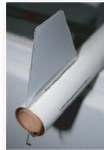
I fabricated the engine mount, and used a Kevlar® cord attachment to the engine mount for the shock cord vs. the standard Estes style shock cord mount. After installing the engine mount, I could begin fin installation. I removed a portion of the protective coating from the polycarbonate and sanded the gluing points. I used 30 minute epoxy for gluing. I used CA at the top and bottom of the fins to hold the fin in place while the epoxy set. I also used 30-minute epoxy for the fin fillets.
