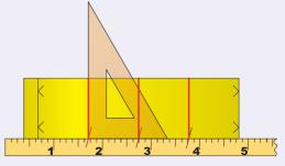
Rewrap the Paper on the Tube and alight the "X" marks. Transfer the lines on the Paper to the Tube.
