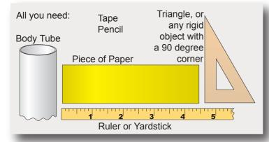
Wrap and Tape the Paper tightly around the end of your Body Tube. Place two "X" marks across the seam. Remove the Paper and lay it flat.
