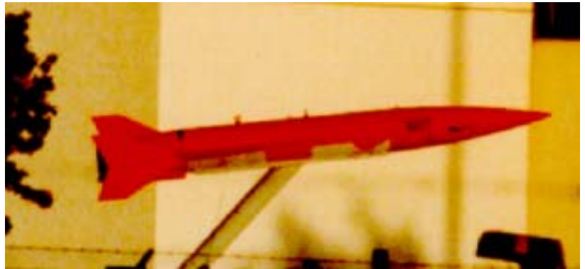
AQM-37A at MSP. The sheet metal appears to be original, but most of the fittings and markings are gone. The flare tube has been cut away to make room for the cradle.
