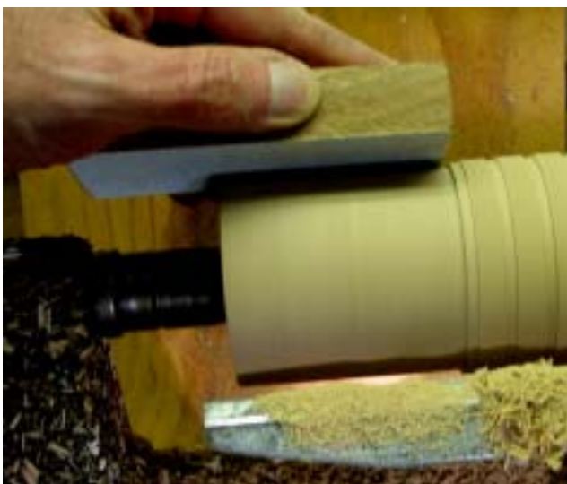
Final sanding of the nosecone shoulder
