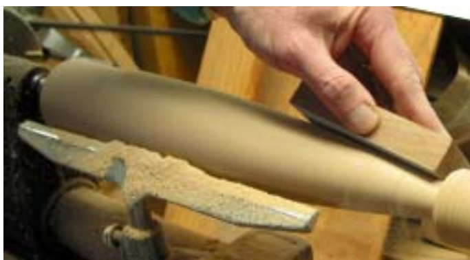
Fine profiling with a sanding block
