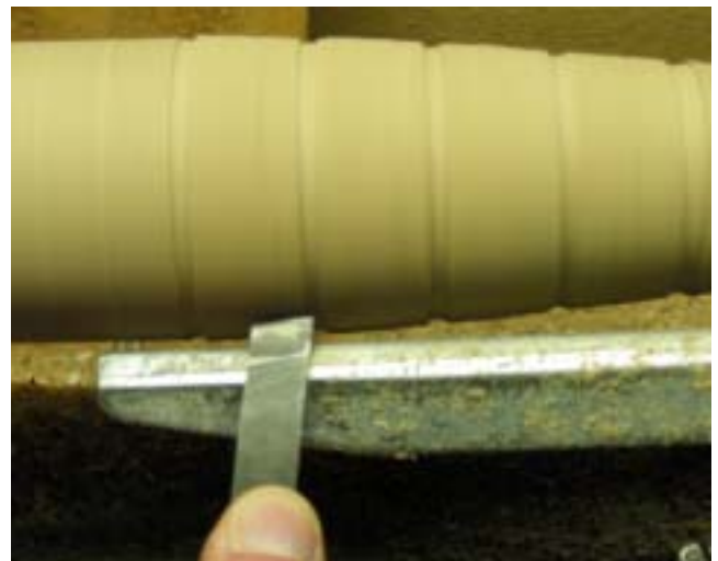
Cutting with the skew chisel -- watch that top profile as you cut!
