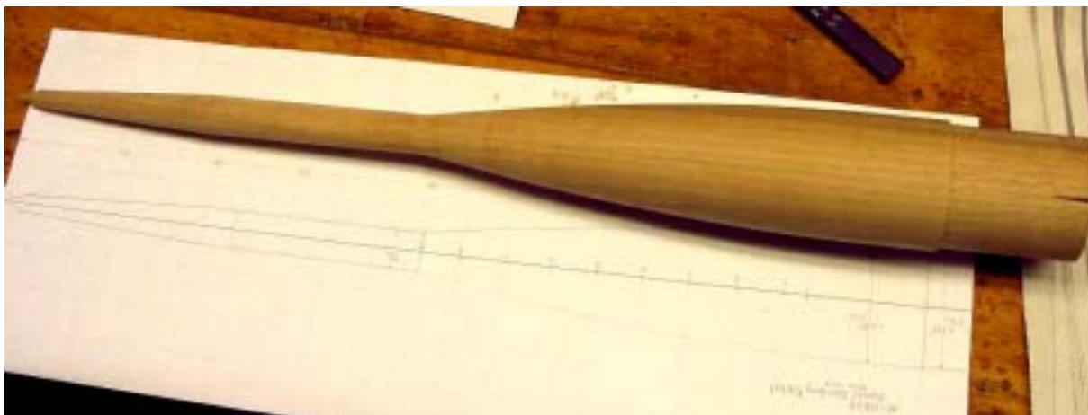
The completed scale M100b nose cone, ready for a 2.6" body tube.
