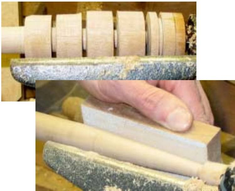
Finishing the taper toward the tip.
