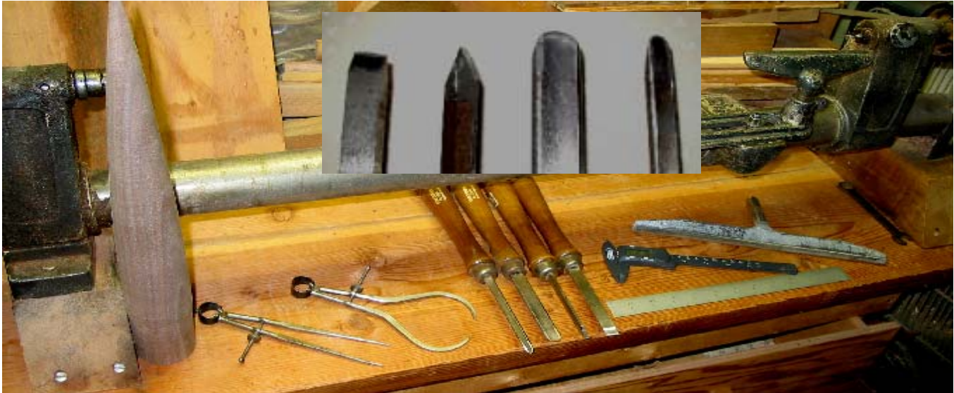
Basic lathe tools (L to R on bench): dividers, calipers, turning tools, dial calipers, steel ruler, long tool rest, Inset: L to R: skew chisel, parting tool, rough gouge, fine gouge.
