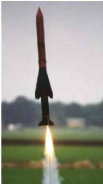
The source of asymmetric thrust is rather easily diagnosed in this memorable flight of Martin Dietl's two (?) motor cluster Exocet last Fall. As this month's *Safety First!* column explains, other causes can be more subtle. (By the way, the Exocet was repaired to fly again by Spring!)
