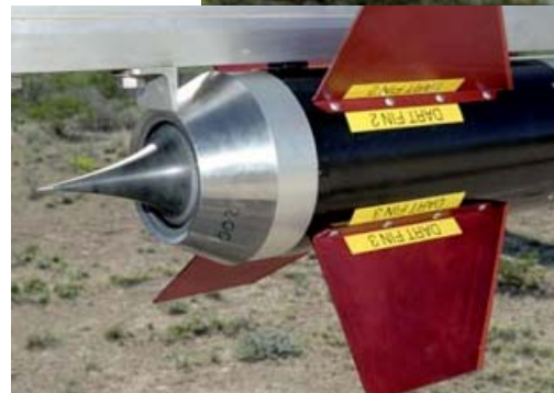
BlackSky and Cesaroni's experimental aerospike nozzle is shown in NASA photos of a successful NASA Dryden test flight in Fort Stockton, Texas. The ten-foot long vehicle reached Mach 1.5 and coasted to over 25,000 feet.
