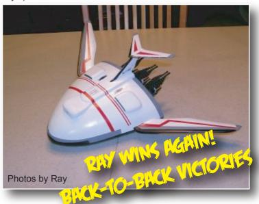
The body of the rocket is 2 vacuum-formed shells with balsa wings (or fins). The substructure is BT20 tubes and balsa supports. The rocket is powered by 3 - 18mm engines which provide enough power to lift it to a nice altitude.
