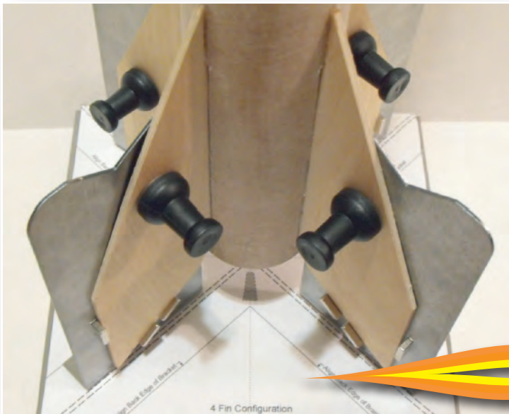
The editor's LOC Tweed-B held in place on the Standard Rockets Assembly Tool
