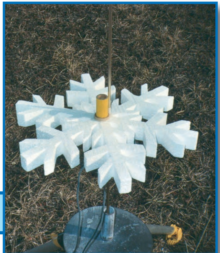
Snowflake from rear view. Shows rear 24mm motor block flush with end of the motor tube and tight against the flake body. The two 24mm motor blocks lock the motor tube tight and perpendicular with the flake body.
