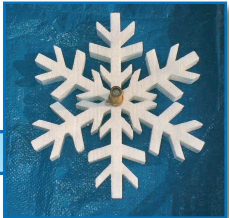
Snowflake from rear view. Shows rear 24mm motor block flush with end of the motor tube and tight against the flake body. The two 24mm motor blocks lock the motor tube tight and perpendicular with the flake body.
