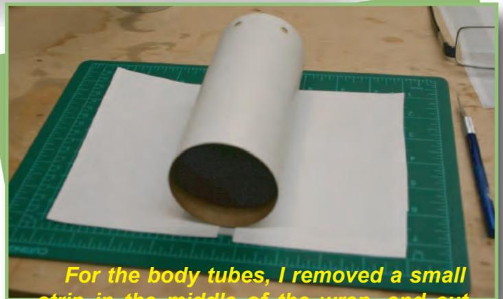
*For the body tubes, I removed a small strip in the middle of the wrap, and cut one edge of the wrap precise to one end of the body tube, and then used a cutting board to ensure that the wrap was square to the tube.*
