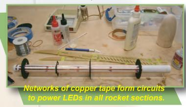
Next is the build-up of the centering rings – making the solder joints small helped when sliding the rings into place. Centering rings were tacked in place with CA, then an engine cover was installed, which had precise slots cut in it to help align the ribs and later the fins. With the ribs epoxied next, it was time to turn to body wrapping.
