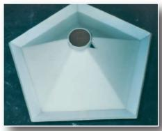
white glue coated. The triangular cut-outs in one side fits a 1/4" rod.
