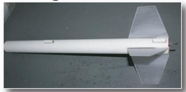
ably due to the epoxy use and also that paint wasn't included in the original analysis, it actually made the model slightly more stable. I then reinserted the actual weight and CG into RockSim and re-ran the engine simulations. This gave me a stability static margin of 1.31 with an E9-6 (the heaviest engine). All other sims were between 1.3 and 1.6.
