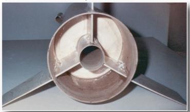
After this internal work is done the rear CTR with motor retaining hardware is test fitted into the body aft end. If the fit is good, I then apply a layer of epoxy to the motor tube, the aft ends of the fin tabs and the adjoining body tube. With one steady push I set the rear CTR in place completing the fin tab cage.
