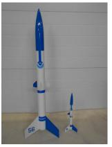
1/8" plywood fins. The lower fins were thru the wall style and the upper surface mount. I obtained the fin patterns thru the RockSim print outs, which made the process very easy. It is fitted with a kevlar/elastic shock cord, 30" chute, and a nomex chute protector. I used a Estes 29mm motor retainer and installed both 1/4" lugs and rail buttons for options on the launch field.
