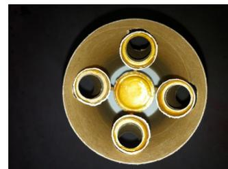
Next I cut the slots in the nose cone shoulder where the motor tubes were, and glued in the nose cone. Then I glued the fincan into the body tube. At this point, if I forgot to do anything inside, I was hosed.
