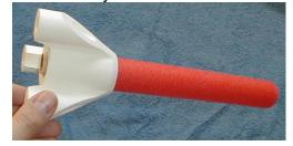
□ 10. Spread glue around the top inside of the white fin unit, on the bottom end and sides of the red body tube, and inside the hole in the red body tube. Glue the red body into the white fin unit. Again, keep a finger on the end of the motor mount tube to make sure it doesn't get pushed out of place. Your rocket is complete! Set it aside to dry overnight before flying it for the first time.
